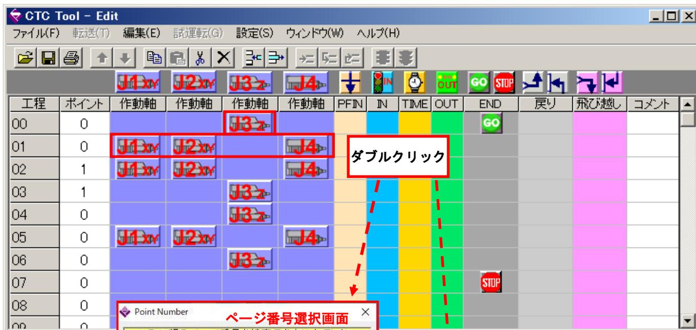
The screenshot shows the 'CTC Tool - Edit' window with a table of program points. The table has columns for '工程' (Program), 'ポイント' (Point), '作動軸' (Active Axis), and various status columns. Icons for J1xy, J2xy, J3xy, and J4 are placed in the '作動軸' column for different points. A red box highlights the J3xy icon for point 00, and a red arrow points to it with the text 'ダブルクリック' (Double-click).
