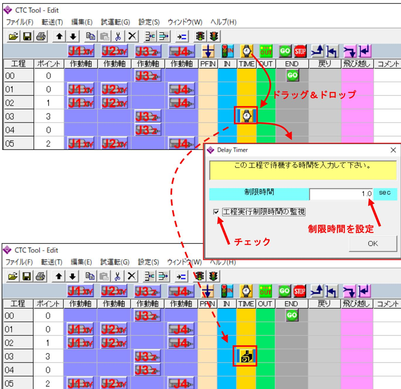
The screenshot shows the CTC Tool - Edit interface with a process table and a 'Delay Timer' dialog box. The process table has columns for '工程' (Process), 'ポイント' (Point), '作動軸' (Axis), 'PFIN', 'IN', 'TIME', 'OUT', 'END', '戻り' (Return), '飛び越し' (Skip), and 'コメント' (Comment). The 'TIME' column is highlighted in yellow. The 'Delay Timer' dialog box contains the following text and controls:
